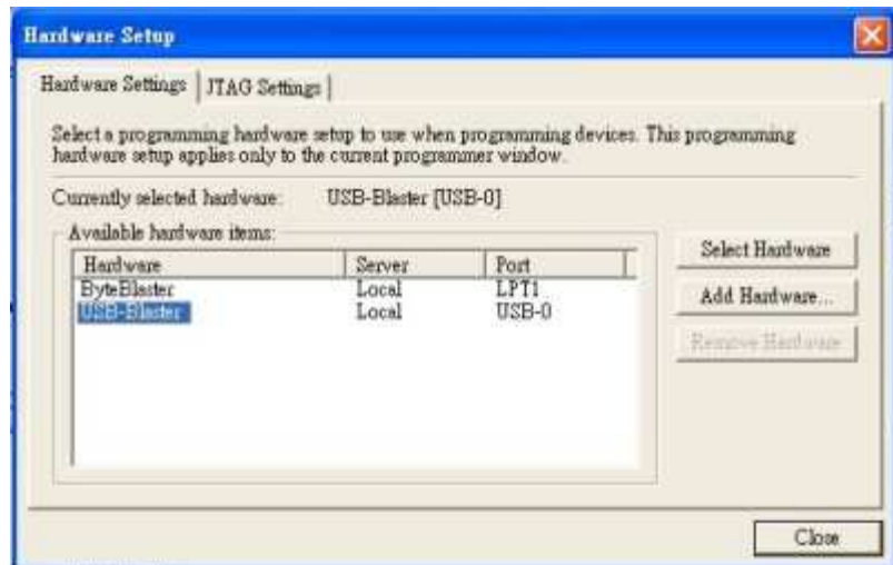
Figure 5.6. Hardware Setup Menu for USB-Blaster
