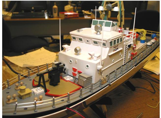
Fig. 4. This R/C toy boat was modified to create a robot boat. PIC microcontrollers, a GPS unit, an electronic compass, a gameboy camera, and a wireless modem are housed inside the cabin. Batteries serve as ballast inside the hull.
