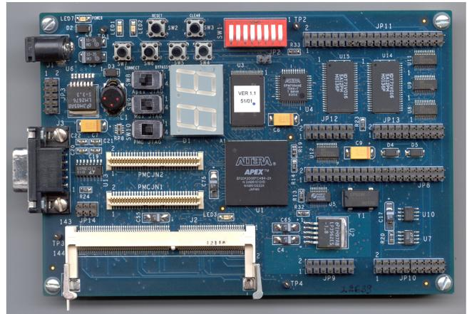
Fig. 11. Altera's Nios SOPC board contains a 200,000 gate FPGA with Flash and SRAM memory. It runs a RISC processor IP core. A C compiler is provided for the processor core. It controls the robots seen in Figs. 6 and 7.
