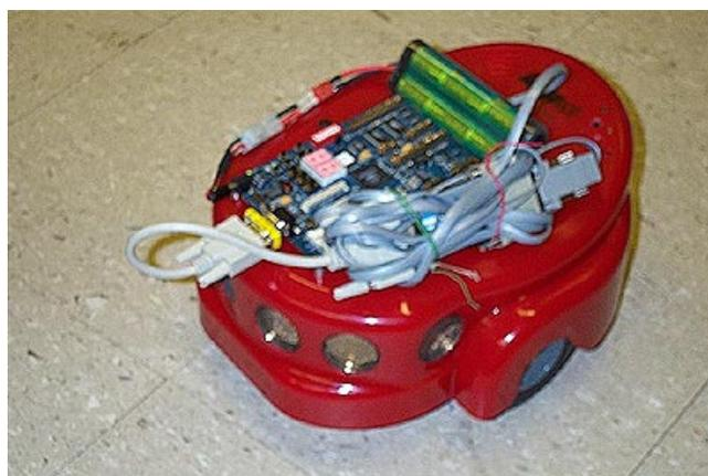
Fig. 7. The small Amigobot commercial robot was originally designed to be remotely controlled using a PC with a serial cable. An FPGA-based SOPC board was added to convert it to an autonomous robot.
