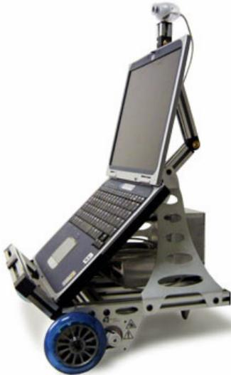
Fig. 8. The ER1 is a commercial robot base designed to carry a notebook PC.
