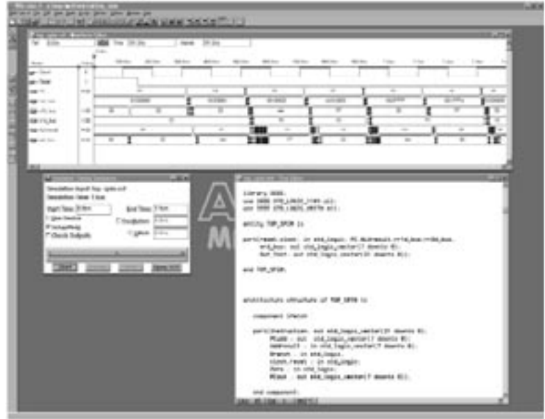
Figure 9. MIPS processor core timing simulation.
