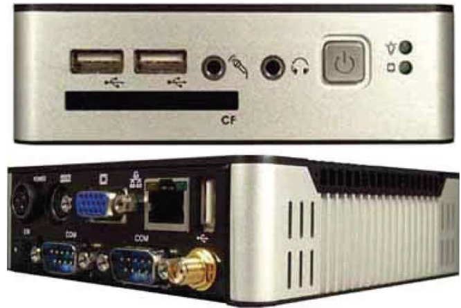
Fig. 1. The 4.5 by 4.5 inch fan less low-cost eBox 2300 X86 SoC computer system has 128 M RAM, 256 M Flash, and all of the I/O features typically found on a desktop PC. Academic pricing is comparable to that of current textbooks ( http://www.embeddedpc.net/academic ).
