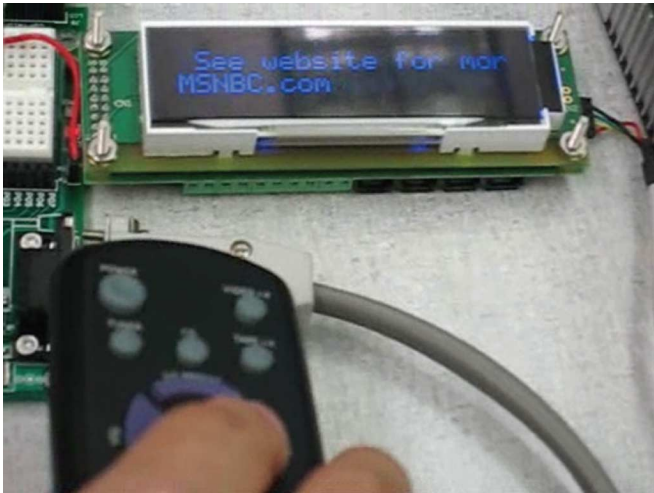
Fig. 6. This project displays scrolling RSS Web news feeds on the Phidget LCD display.
