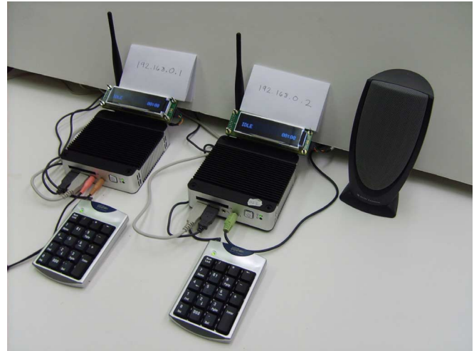
Fig. 7. A student VoIP Phone system project using two eBoxes.
