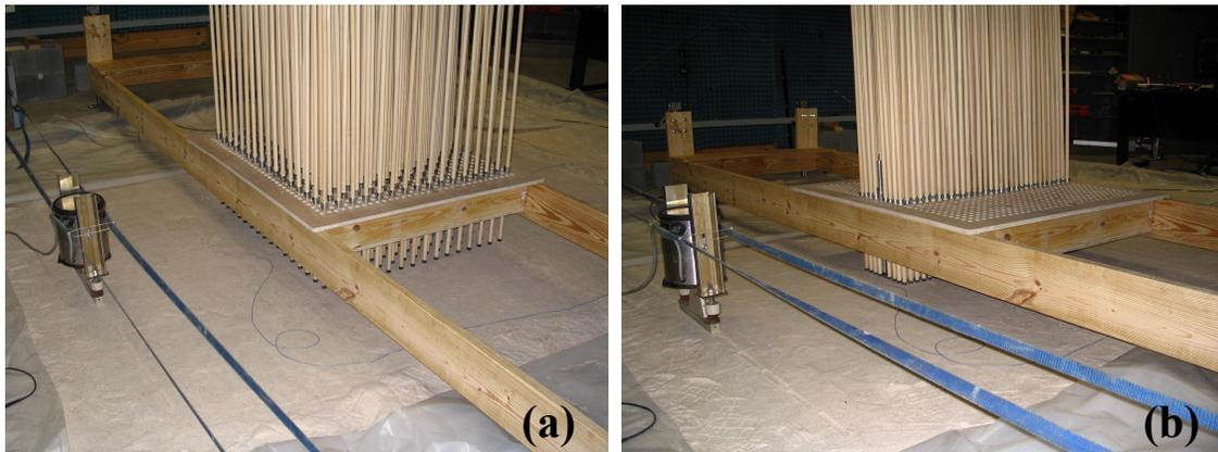
Figure 3: Laboratory Experiments on Ground Loading by Large Arrays of Sensors with (a) 16 by 16 Array of Mock Sensors Covering  $1\text{ m}^2$  and (b) 9 by 32 Array with One Line of Ground-Contacting Sensors.
