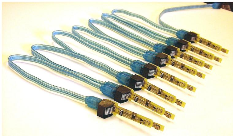
Figure 7: Row of Daisy Chained Sensor and 16-bit A/D PCBs.
