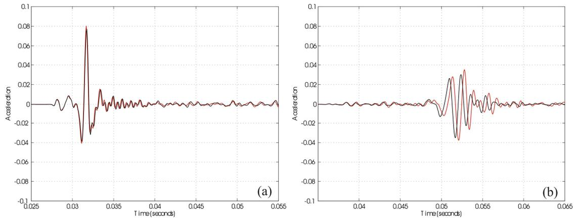
Figure 4: Normal Surface Acceleration With and Without Ground Loading of 16 by 16 Array of Mock Sensors Covering  $1\text{m}^2$  (a) in Front of and (b) Behind Array Location (Red lines indicate data without ground loading while black lines indicate data with ground loading).
