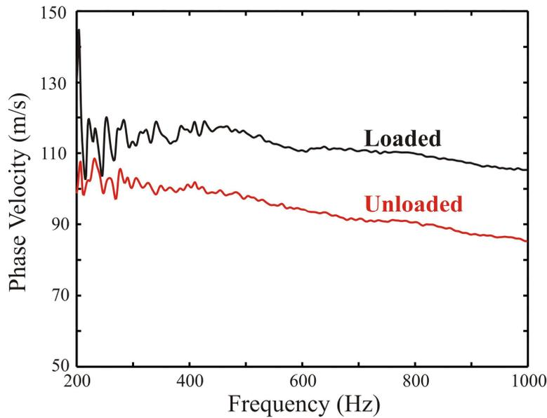
Figure 5: Phase Velocity of Rayleigh Surface Wave With and Without Ground Loading of 9 by 32 Array with One Line of Ground-Contacting Accelerometers Along the Centerline of the Array.
