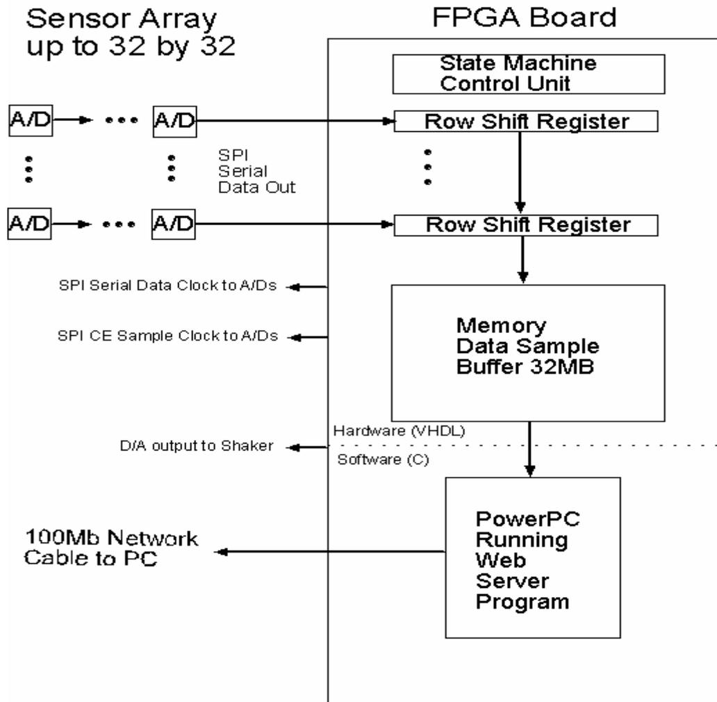
Figure 6: Block Diagram of Data Acquisition System.
