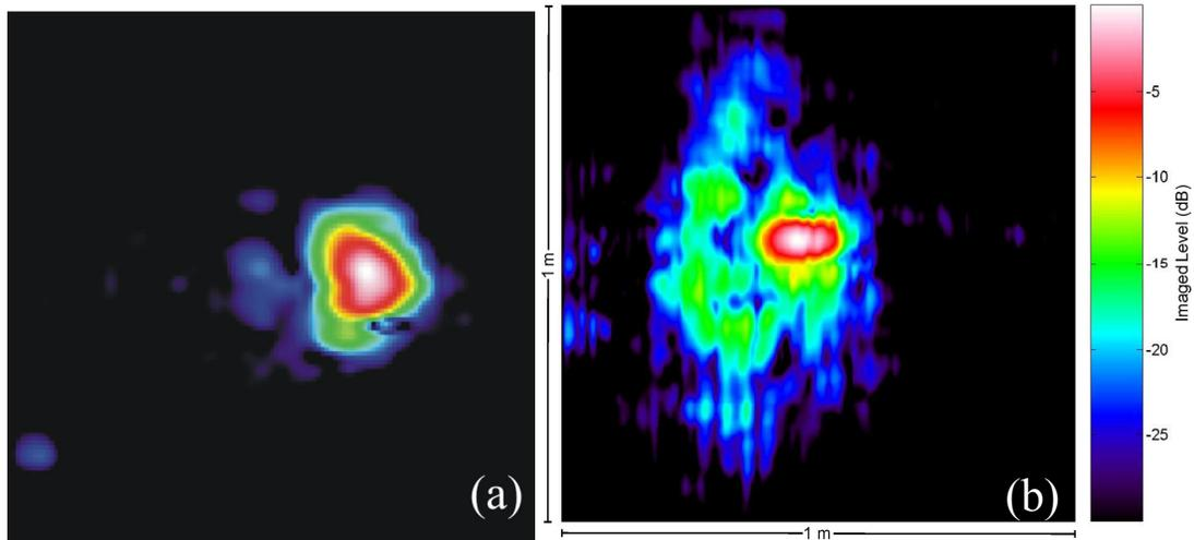
Figure 2: Images from Field and Laboratory Experiments with Ground-Contacting Accelerometer Sensors with (a) 32-Element Linear Array over a  $1\text{ m}^2$  region with a VS-2.2 AT Landmine at a U. S. Government Test Facility and with (b) a Single Sensor Scanned over a  $1\text{ m}^2$  region with a VS-1.6 AT Landmine Buried 8 cm Deep in the Experimental Model at Georgia Tech.
