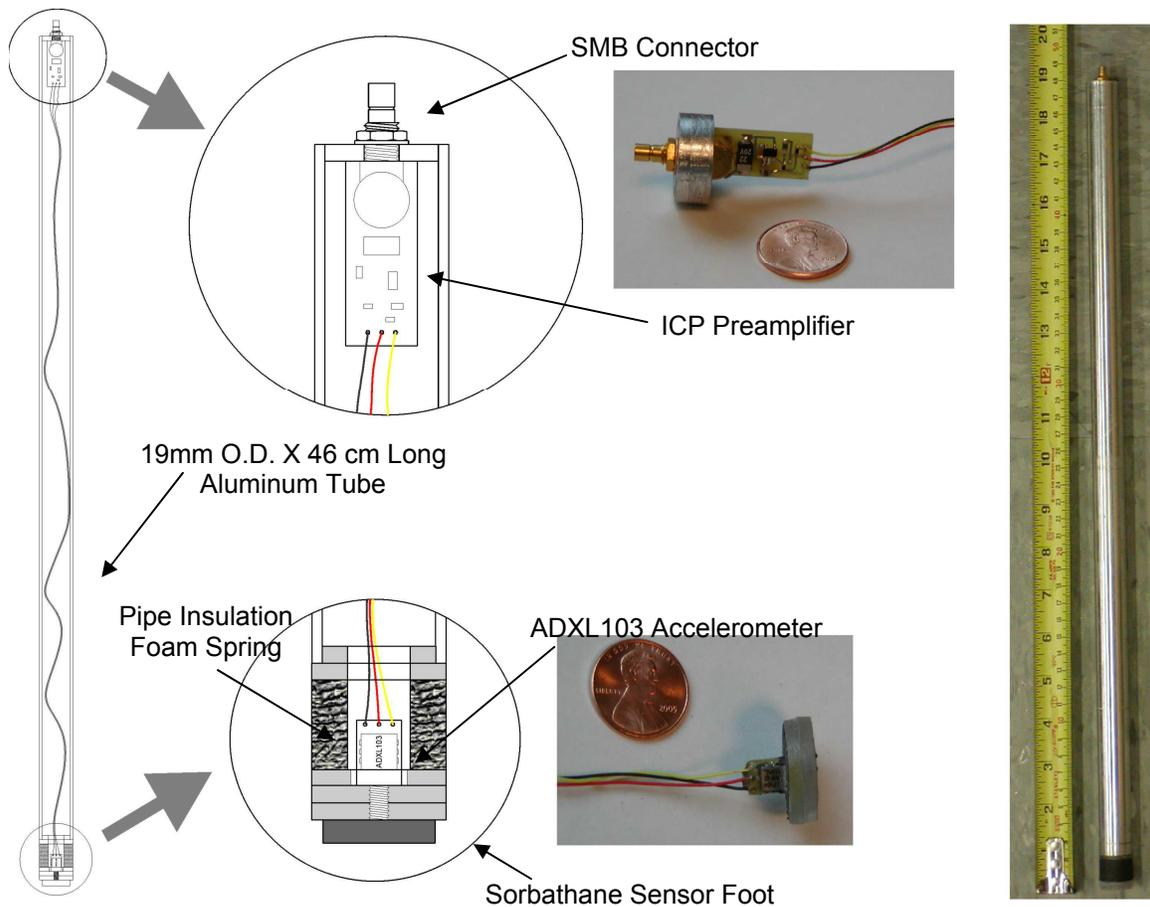
Figure 1: Ground-Contacting Accelerometer Sensor Photographs and Drawings.
