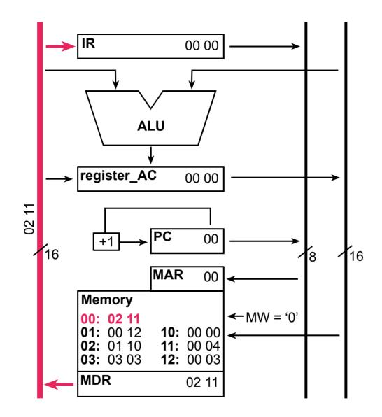
Figure 9.7 Datapath used for the µP 3 Computer Design. Values shown after applying reset.
