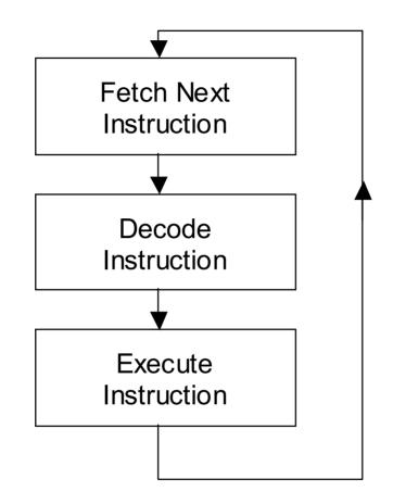
Figure 9.5 Processor Fetch, Decode and Execute Cycle.
