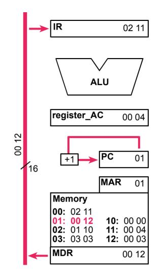
Figure 9.8 Register transfers in the ADD instruction's Fetch State.
