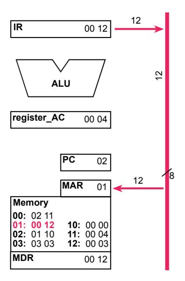
Figure 9.9 Register transfers in the ADD instruction's Decode State.
