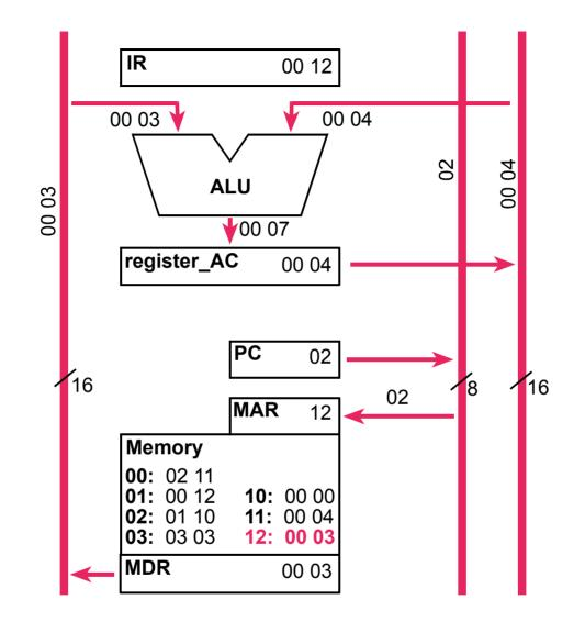
Figure 9.10 Register transfers in the ADD instruction's Execute State.
