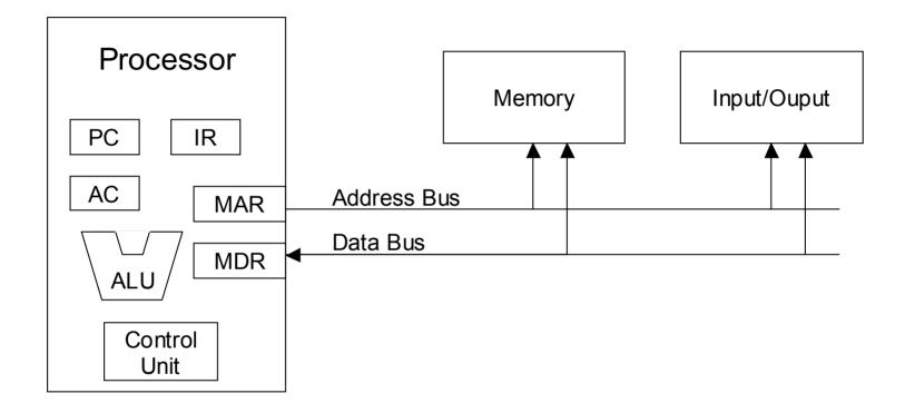
Figure 9.1 Architecture of a Simple Computer System.
