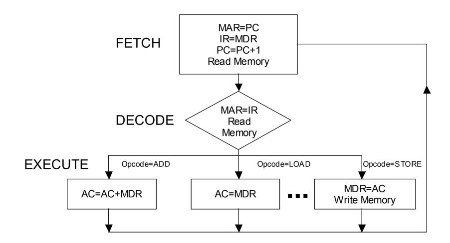
Figure 9.6 Detailed View of Fetch, Decode, and Execute for the µP 3 Computer Design.
