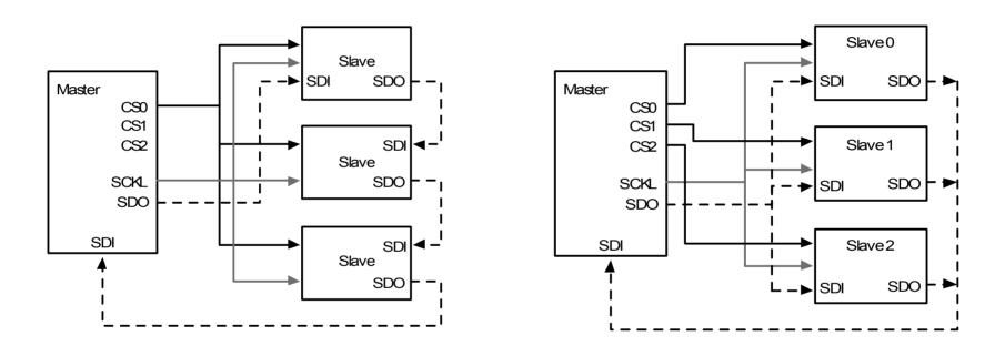
Figure 12.3 The two SPI slave device configuration options.
