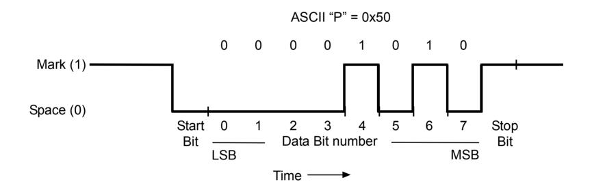
**Figure 12.2** RS-232C Serial interface transmission of an 8-bit data value
